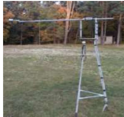
← Wilson antenna at Świder for measuring electric current density
