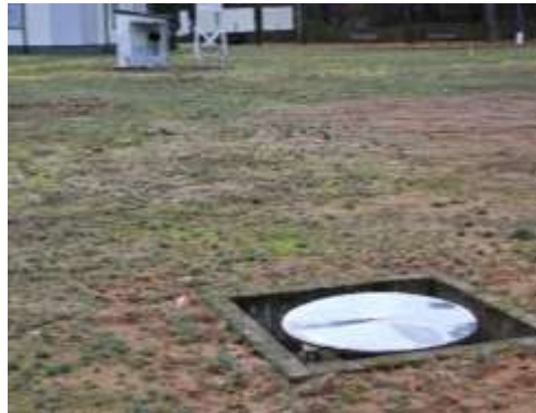
← Wilson antenna at Świder for measuring electric current density
